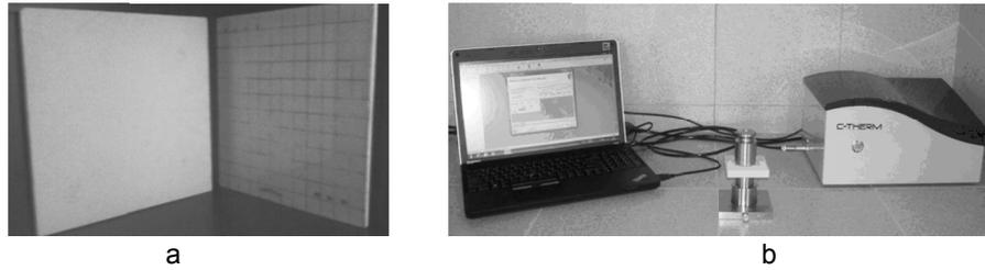
Fig. 1 General view of a testing specimen (a) and of the TCi analyzer (b)
