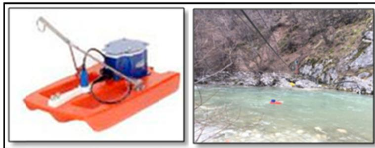
Fig.9 Teledyne RD Instruments Stream Pro ADC
