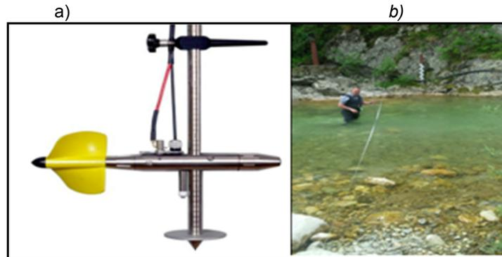
Fig. 5 Universal current metering Wing F1
