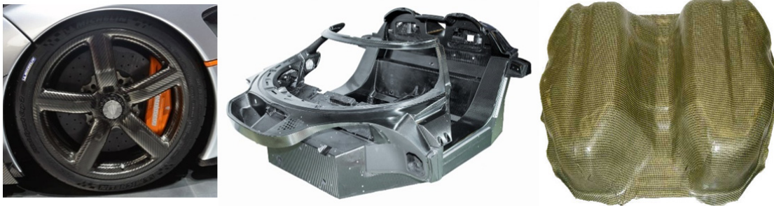
Figure 9: Carbon fiber wheel, Carbon fiber tub, Kevlar fuel tank
